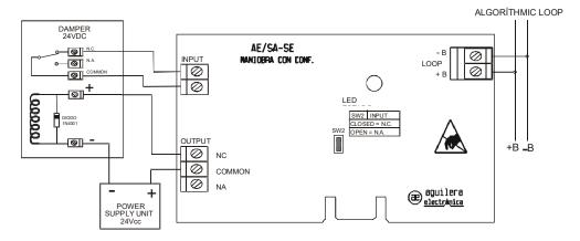
A damper has been shown that needs to be continually fed. If it is desired to connect a damper that needs voltage to close, the positive of the solenoid valve has to be connected to the normally open (NA) contact of the module output.
